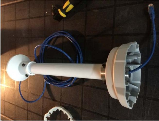
8) Now connect the patch cable sticking out from the hole in the UMA/Pendant cap, into the Ethernet jack on the camera & attach the camera to the pendant cap & replace the dome.
