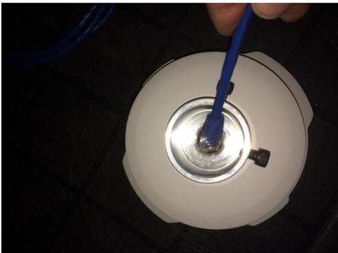
7) Attach the UMA/pendant cap to the open end of the tube.
